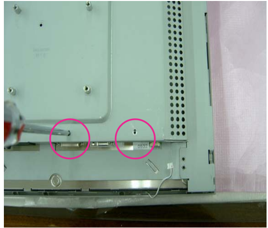
3. Separate cable Main Board and Separate screw between Shield PCB and Bracket PCB.(2 point)
